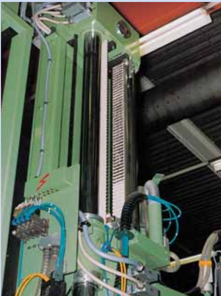
Siegling Proposition timing belts in the vertical axis of an industrial robot.
