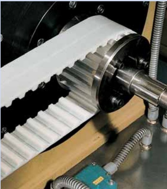
Siegling Proposition on the power test rig.
