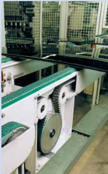
Conveying of car windows by belts running synchronously. The coverings on the reverse face of the timing belts treat the goods gently and improve the grip properties.
