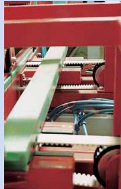
Conveying of car windows by belts running synchronously. The coverings on the reverse face of the timing belts treat the goods gently and improve the grip properties.
