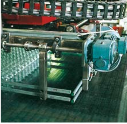
Modules with a smooth surface make accumulating and palletizing bottles on the conveying line possible.
